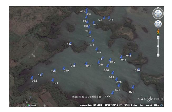
The average water depth recorded was 2.1m. The deepest point recorded was 3.6m at locations # 35 and 36, while the shallowest point was observed at locations # 51 and 52 for a depth of 0.7m. From locations # 31 to 37, the average water depth recorded was 3.4m.
